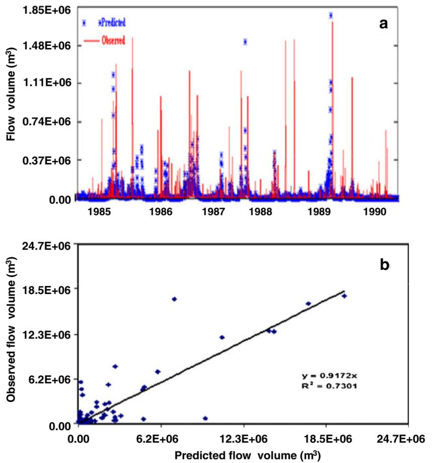
**Fig. 3** Comparison of predicted and measured water flow (a) and flow volume (b) during validation process
