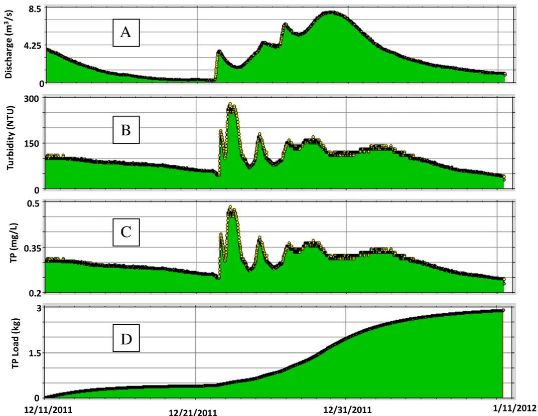
Fig. 4. Real-time variations of discharge (A) and turbidity (B) measured by USGS and real-time variations of TP concentration (C) and load (D) predicted from the DDDAS for a 30-day monitoring period from December 11, 2011 through January 10, 2012.
