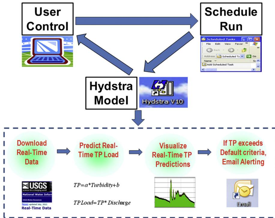
Fig. 2. A dynamic data driven application system for monitoring real-time variation and load of TP in surface waters.
