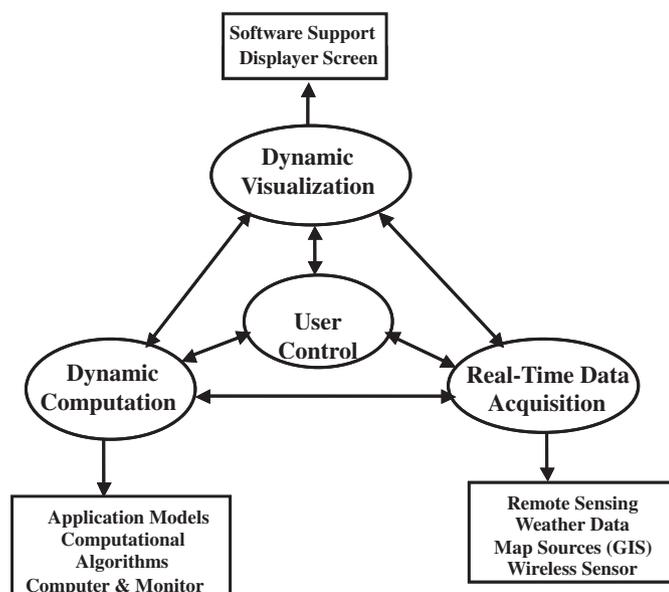
Fig. 1. A schematic diagram showing the basic concept of a dynamic data driven application system redrawn after NSF (2000).
