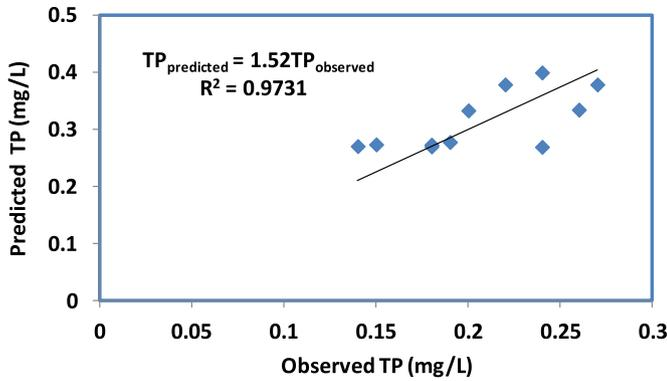
Fig. 3. Comparison of field measurements and DDDAS predictions for TP concentrations.
